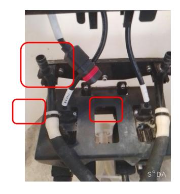
Do not allow water to penetrate the pins on the peristaltic pump.
