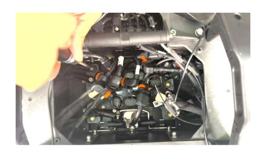
We check the screws at the 4 ESC power positions on the main control circuit. Test cycle is once a week (Time may vary depending on machine operating capacity)
