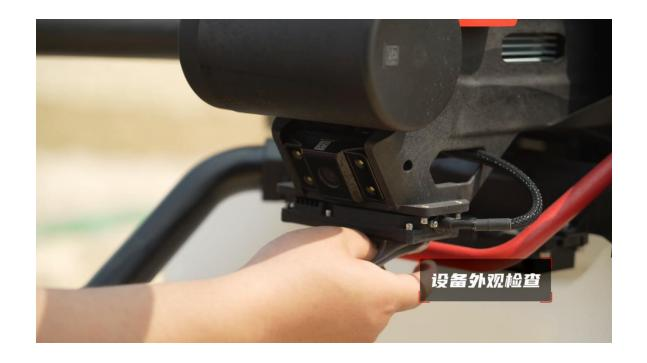
Clean the surface of the terrain radar to make the altitude scanner accurate
