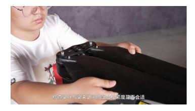
Check the tightening of the propeller screws, the propeller after tightening the screws will have a moderate stiffness when we open / close by hand, the two sides of the wing must have the same stiffness.
