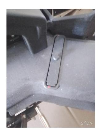
We remove the rubber cover and proceed to check the tightness of each arm clamping screw.
