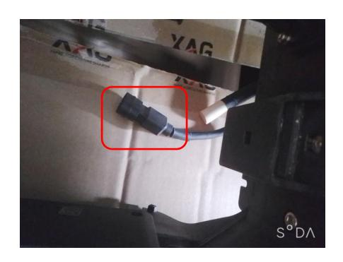
Do not let water get inside the spray/spray tank connection wire on the body
