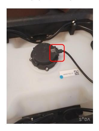
Clean regularly and avoid spilling water on the sensor on the spreader/irradiator.
