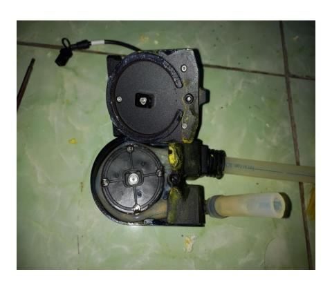
Apply vaseline for the position of the peristaltic pump in the pump after about 60 ha for rice.
