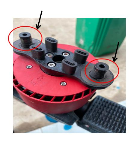
After a period of use, the wing friction with the shaft leads to the stiffening of the wing. When the wing rotates, the arm vibrates strongly.
